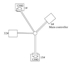
In such circumstances the factory recommends the usage of RS485 distributor. The distributor can change the star configuration connection to the mode of connection stipulated in the RS485 standards. The new connection achieves reliable data transmission. (Refer to Picture 9-6.5).
