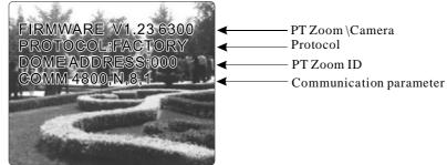
The information will not disappear until you stop to operate the system. If you set "power up action", the dome will automatically activate motions after self-testing. How to operate the function? We will explain detail introduction in following passages.
