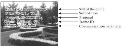
The information will not disappear until you stop to operate the system. If you set "power up action", the dome will automatically activate motions after self-testing. How to operate the function? We will explain detail introduction in following passages.
