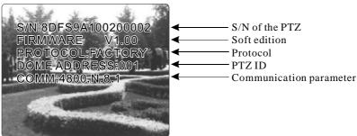
The information will not disappear until you stop to operate the system. If you set "power up action", the PTZ will automatically activate motions after self-testing. How to operate the function? We will explain detail introduction in following passages.
