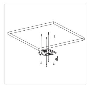
1.To drill 4 M4 screw hole in ceiling (see above sketch), use 4pc STP4X16 cross screws to fix the upside-down installation board of D57 on ceiling.
