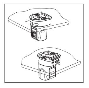
4.Use 3pcs M3X5 cross screws to fix the connection board and installation board, like above sketch.
